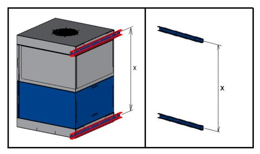
• Put the filter unit with its wall brackets on the wall brackets attached to the wall and screw them by means of the delivered screws.
